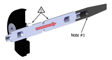
Note #1 - Shaft fitting tool included in spares kit DXK-4 This must be used when re-fitting centre shaft
